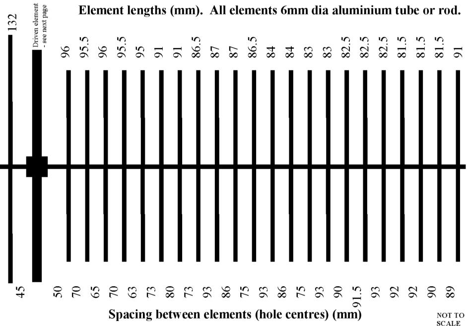
Boom material: 15mm square section aluminium, length approx 1950mm
