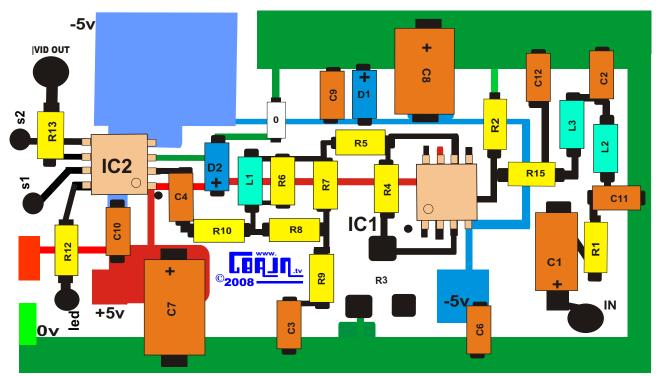
IC2 pad must make electrical contact to negative line.
